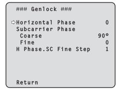
5 Press the [▲] or [▼] button to bring the cursor to "Horizontal Phase", and press the [○] button.
